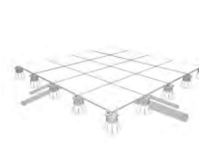
3. Elements such as pipes are completely hidden under the panels.
