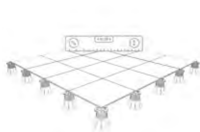
9. Flat and level finish. Slopes and drains are hidden.
