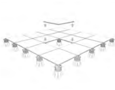
2. Panels can be lifted anytime, granting permanent access to the subfloor.
