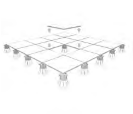
2. Panels can be lifted anytime, granting permanent access to the subfloor.
